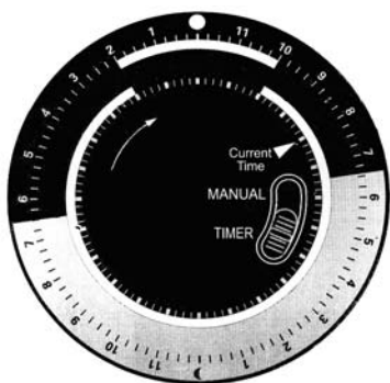
Figure 8- shows timer set to turn appliance ON at 10 AM and OFF at 2 PM. Notice ALL segments between 10 PM and 2 AM have been pushed out. Current time is 8:00 AM.
